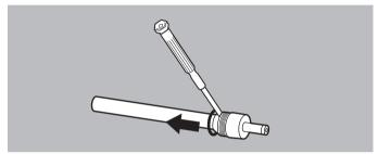
2. Remove the sealing ring carefully with a screwdriver, without damaging the groove.
