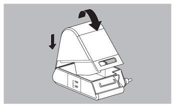
10. Place the top of the humidifier on the base of the humidifier from the back and press down gently until it clicks into place.
