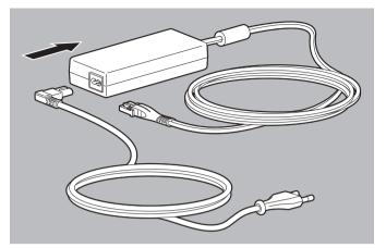
1. Connect the power supply cable with the power supply unit.
