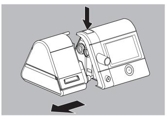
2. The respiratory air humidifier is removed from the side of the therapy device.
