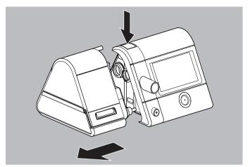
3. The respiratory air humidifier is removed from the side of the therapy device.
