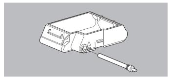
1. Unscrew the element from the base of the humidifier.
