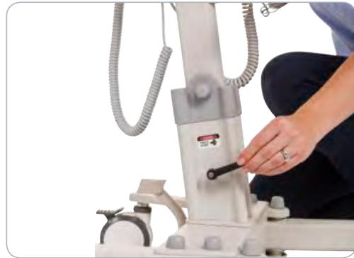
6. Fold mast down carefully and secure to legs with cords located under the end of legs.
