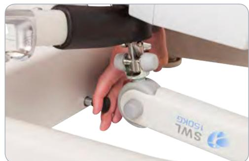
5. Undo base fastening lever bolt and remove bolt.
