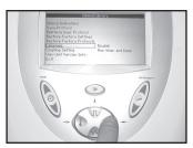
3. Press the DISPLAY (enter) button to accept the highlighted selection.
