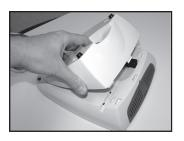
6. Replace the mounting bracket on the back of the unit.
