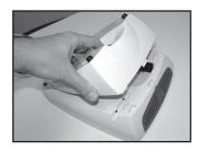
1. Remove the mounting bracket from the back of the unit.
