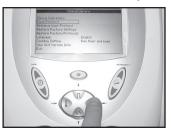
3. Press the DUTY CYCLE (up arrow) and FREQUENCY (down arrow) buttons to highlight Save Protocol, and press the DISPLAY (enter) button to accept the highlighted selection.
