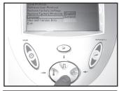
4. Press the FREQUENCY (down arrow) and DUTY CYCLE (up arrow) buttons to highlight the appropriate language.
