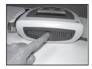
To brighten or dim the LCD, turn the contrast control dial until the display contrast is optimal.
