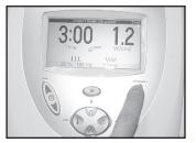
5. Press the Intensity button and raise or lower the unit's output using the up and down arrows.
