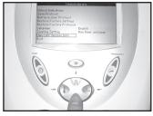
2. Use the FREQUENCY (down arrow) and DUTY CYCLE (up arrow) buttons to highlight the View User Info option.
