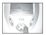
3. Press the DISPLAY (enter) button to accept the highlighted selection. The Restore Factory Protocols Confirmation window displays.
