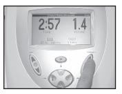
6. Press the START button. The unit will beep 5 times and the ultrasound power will distribute the selected output.
