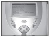
3. Press the FREQUENCY (down arrow) or DUTY CYCLE (up arrow) buttons to highlight the Save Protocol option.
