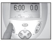
2. To make INTENSITY and treatment TIME changes, touch the respective buttons and use the up or down arrows to advance to the desired settings.
