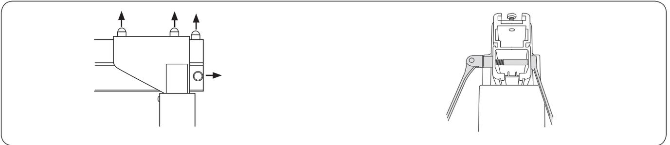
3. Remove the cover caps from the screws on the corner/locking rail and stop bolt on one end of the rail.
