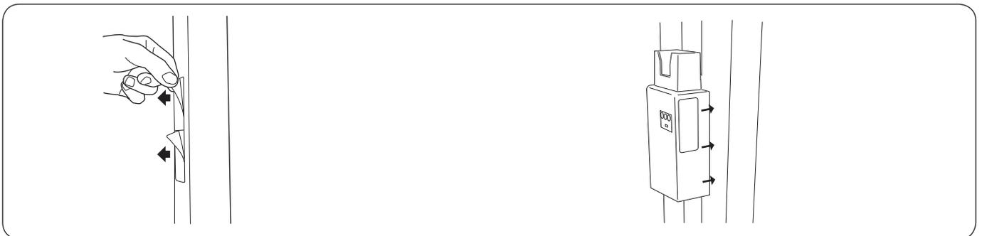
Remove the protective film from the double-adhesive tape (on the inner side of one of the upright supports).
